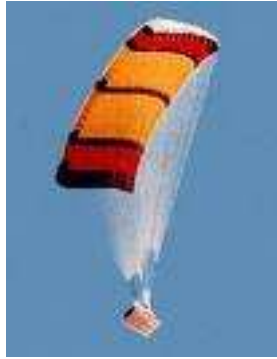
Figure 2.3: Parafoil used to deliver cargo [SEC07].
