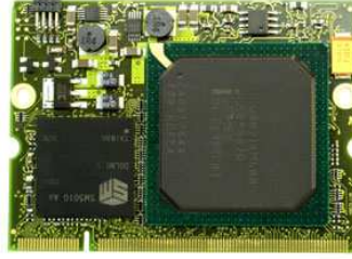
Figure 2.11: Kontron's GP8 X-Board. Large chip on dominating right side of board is the Intel 80219 CPU. Smaller chip on left is the SM501 Graphics chip [KON06].
