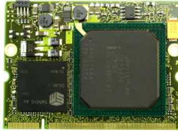
Figure 3.9: The Kontron GP8 is a general processing module which utilizes the Intel 80219 ARM architecture to deliver 600MHz processing. In addition, the GP8 module also has an on-board SM-501 graphics chip to provide SVGA video output capability [KON06].
