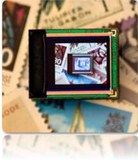
Figure 2.7: Size of OLED compared to postage stamps. OLED is utilized by STS in their AN/PVS-21 LPNVG HUD system [STS07].
