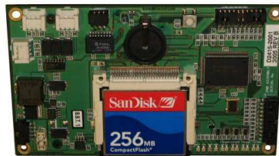
Figure 3.11: This photo shows the rear of the D2426 with an inserted CompactFlash card, plus the external mount points [INT07b].
