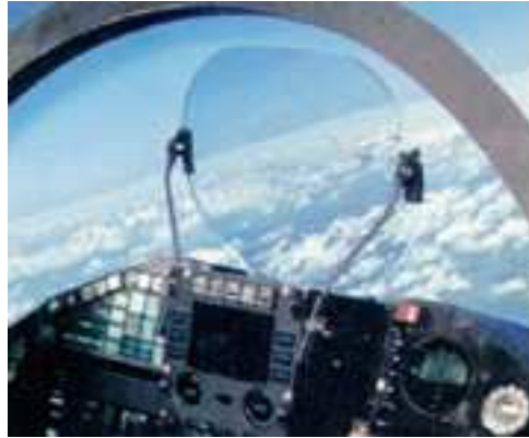
Figure 2.5: F-22 HUD example; standard HUD currently utilized in military aircraft [QSA08].
